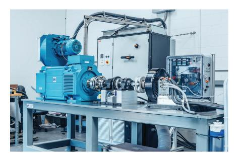
ORIGINALLY DESIGNED FOR THE DEVELOPMENT OF THE X-57 MAXWELL, this dynamometer is uniquely capable of characterization of hybrid and electric drivetrains for aircraft certification. The EDS300 is a stand-alone system essential for Advanced Air Mobility development. The EDS300 system also regenerates power from the test article, significantly reducing facility needs and the energy consumed during testing.
