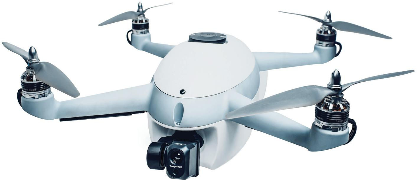
FAST-ISR is designed for advanced air operations by a single user. Coming standard with a payload release kit, FAST-ISR can also be equipped with alternative payloads such as munitions and electronic warfare devices. FAST-ISR differs from its predecessor with the integration of FLIR's Hadron 640R electro-optical and infrared camera paired with a nose mounted 2-axis gimbal.
