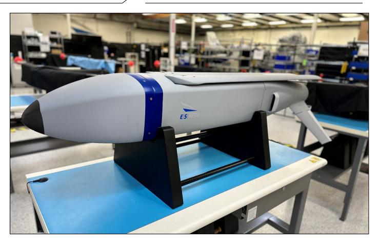
Lumberjack is a Group III unmanned aircraft designed to overcome the tyranny of distance by being launched from ground systems or air vehicles. This vehicle can deliver enhanced lethality to multiple locations through a low-cost logistically flexible platform.
